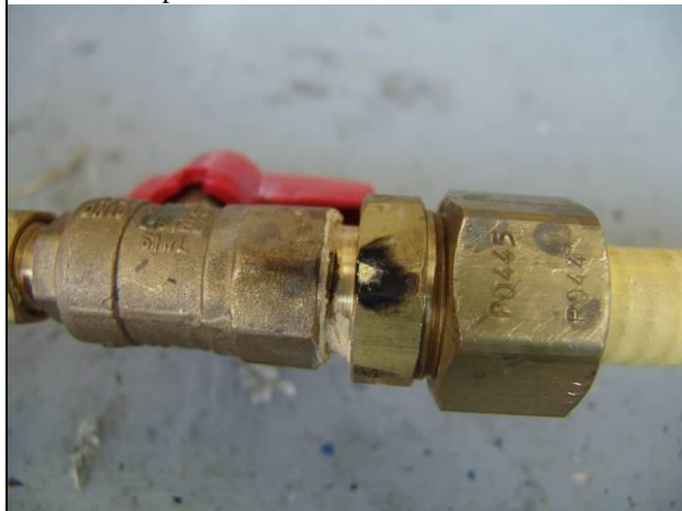
Figure 4: Charge is transferred at heavy wall
