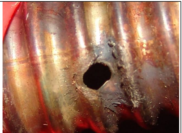
Figure 5: Charge exit at thin wall
