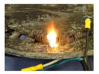
As the wire became hot, the insulation began to smoke, which is evidence of rapid off-gassing. Then the PVC flashed and free-burned. Just prior to ignition, a spark was observed. A spark is consistent with electrical faulting. The hot-wire operated at a temperature of approximately 400°C and a power intensity of approximately 39 W/cm.
