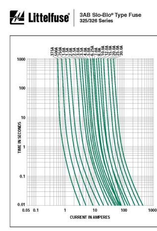
Since a short circuit is considered to be 6 times the rated current, the circuit impedance is reduced to 1 Ohm. Under that fault condition, the fuse will blow in about 0.07 seconds.
