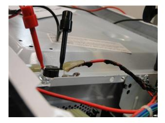
The location and orientation of a TCO is critical to its performance. Otherwise, adjacent burning can occur with no impact on the flow of the electrical circuit as seen in the photo.
