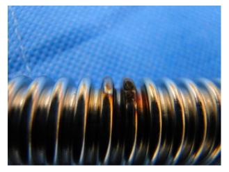
Based on calculations shown, the corrugated tubing is penetrated by electrical energy much more easily than alternative piping systems.
