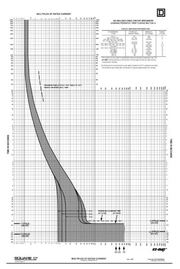
A standard 120 Volt, 20 Amp circuit breaker will run continuously at 20 Amps. The breaker asymptotically approaches its rating above 300 seconds. The available energy through the breaker is calculated at 300 seconds but in reality is infinite, since the breaker will not trip.
