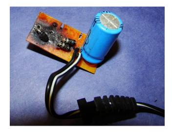
The low-end amount of power required to create ignition varied from about 12 to 22 watts at voltages in the 9-15 volt range.
