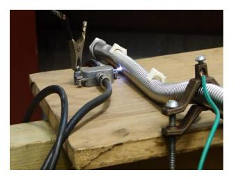
The area is related to the radius of curvature at the ridge versus the radius of curvature of the cylindrical pipe. The nominal external radius of the corrugated ridge is .04", while the nominal radius of 1/2" steel pipe is 0.42", which is greater than a factor of 10.
