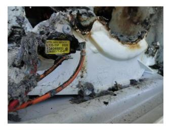
Another appliance TCO was evaluated. The device has a nominal rating of 100°C. Direct flame was applied to the connector insulation, which melted and burned. The TCO did not open the circuit.
