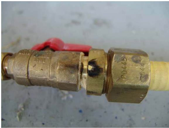
Fig. 4. Charge is transferred at a heavy wall.
