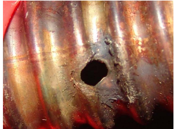
Fig. 5. Charge exit at a thin wall.
